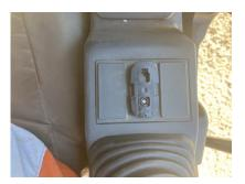
Image Comment(s):Coupler control switch missing cover.
